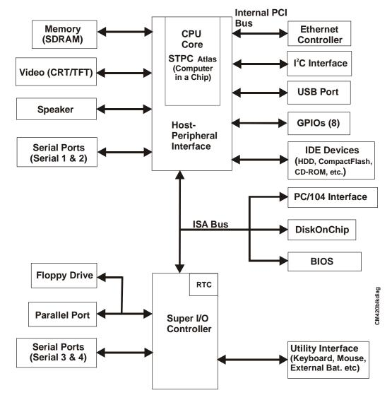
Figure 2-2. CoreModule 420 Block Diagram
